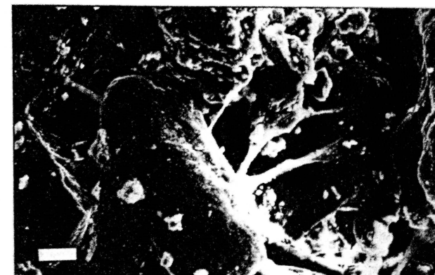
Figure 5. Silt-sized quartz grain bound to the crust by polysaccharide threads derived from a cyanobacterial sheath (bar = 0.01 mm).
